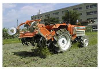
Fig. 3 Tractor with Rotary Tiller
