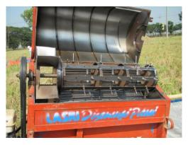
and axial flow thresher shown in Fig 12 has been widely used in Southeast Asia. In 1990s a combine equipped with this type thresher has been developed. Both threshers for indica and japonica rice are originally designed for rice threshing.
