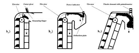
Figure 1. Systems for continual crop yield volume and mass flow determination
