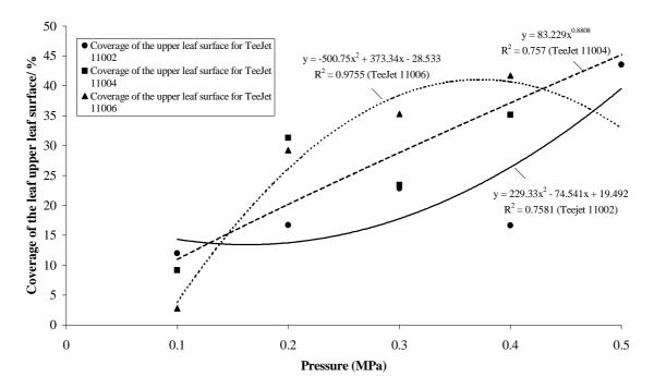
Fig. 7. Coverage of the upper leaf surface for three nozzle types depending on the spraying pressure
