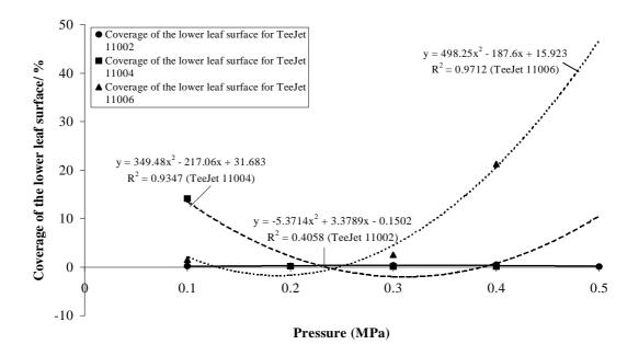
Fig. 8. Coverage of the lower leaf surface for three nozzle types depending on the spraying pressure
