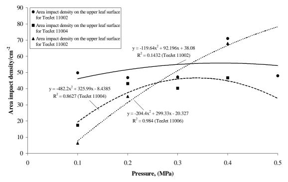
Fig. 9. Area impact density on the upper leaf surface for three nozzle types depending on the spraying pressure
