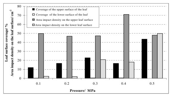
Fig. 4. Average coverage and area impact density on the upper and lower winter wheat leaf sides in case of the use of TeeJet 11002
