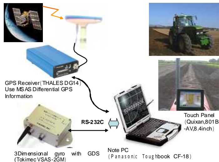
Fig.1. Standard guidance system hardware construction
