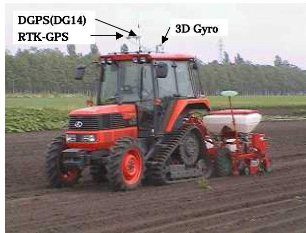
Fig.7 Field experiment using the guidance system
