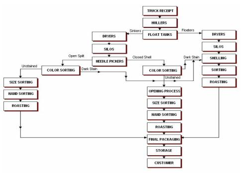
Fig. 1. Diagram of pistachio process steps in California (Vincent Corp 2007).
