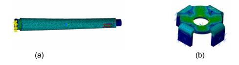
Fig. 6. stress distribution of Von Misses in sensitive components of the machine: (a) Shaft, (b) Shaft support.
