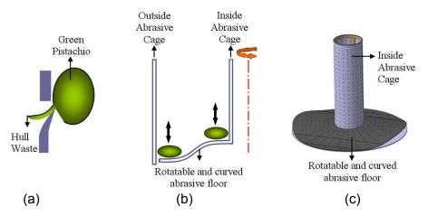
Fig. 3. Schematic view of the working principles of pistachio multipurpose machine: (a) hull removing method, (b) hull removing principles, (c) Inside abrasive cage and curved bottom
