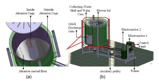
Fig. 2. General view of the proposed multipurpose machine: (a) Machine process chamber, (b) Different parts of the machine.
