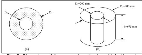
Fig. 5. Dimensions of the processing chamber: (a) inside and outside abrasive cages, (b) Rotatable and curved abrasive bottom.
