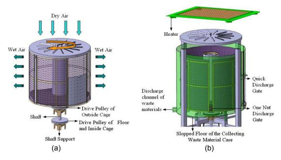
Fig. 4. (a) Drying operation method, (b) Different discharge channels.
