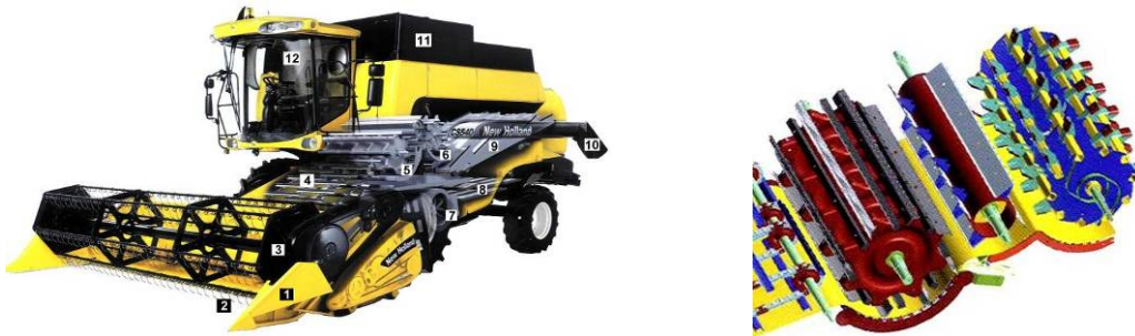
Fig. 8 - Combine harvesters NEW HOLLAND CS540 system and threshing / separation [2]
