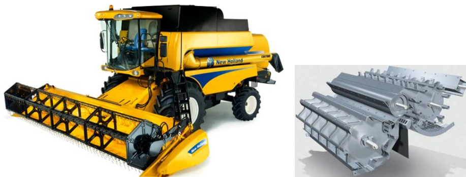
Fig. 9 - Combine harvesters NEW HOLLAND CSX 7080 system and threshing / separation [2]
