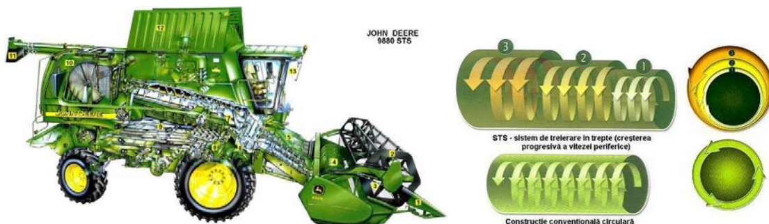
Fig. 7 - Combine harvesters JOHN DEERE 9880 STS and threshing machine [1]
