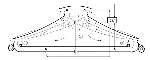
fig.3. Energy loop of energy-economical livestock building for floor breeding of animals and birds (patent [6])(TP –thermal pump, 1 – feeding channels, 2 – sucking channels, 3 – feeding facilities, 4 – bio generator chambers)
