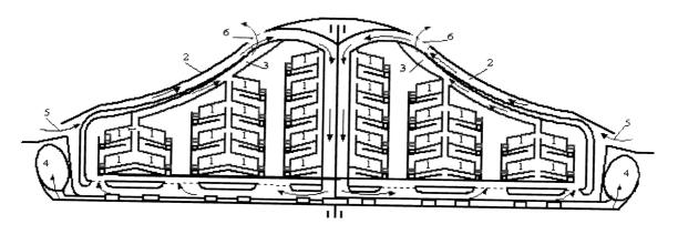
fig.4. Energy loop for cage bird breeding (patent [7] ) 1 – cages; 2 – fresh air feeding channels; 3 – channels for removal of polluted air; 4- bio gas chambers; 5 – feeding openings; 6 – vent.
