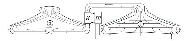
fig. 7. Energetical and manufacturing compatibility of the loops (1 – drying chamber, 2 – livestock building, TP – thermal pump, E – evaporator, K - condenser)
