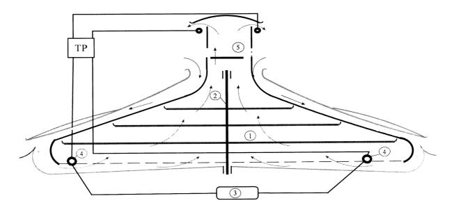
fig.6. Configuration and specific parameters for energy loop for fruit and vegetable dryer (patent [8]) (TP – thermal pump, 1 – working chamber, 2 – carrying axis and grids, 3 – boiler, 4 – heating serpentine)
