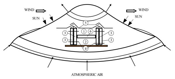
fig.2. Initial surface and modular element for loop formation (1 – feeding (incoming) channel , 2 – sucking channel , 3 – carrying frame, 4 – attachment bolts, 5 – roof element, 6 – insulating layer)
