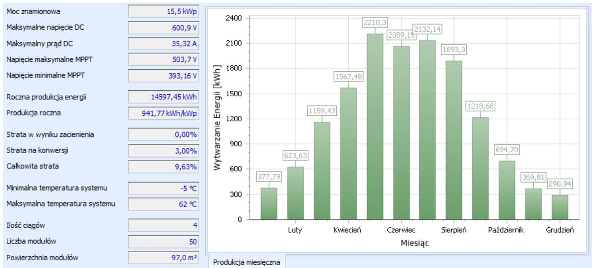
Fig. 6. Performance and the number of selected monocrystalline panels [source: own calculations in BlueSol].
