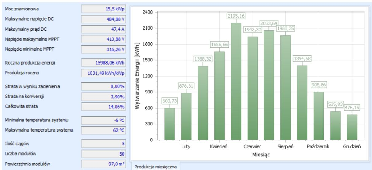
Fig. 5. Performance and the number of selected polycrystalline panels [source: own calculations in BlueSol].
