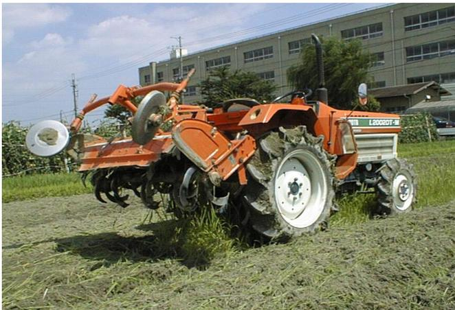
Fig. 3 Tractor with Rotary Tiller
