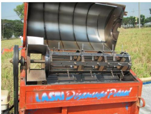
and axial flow thresher shown in Fig 12 has been widely used in Southeast Asia. In 1990s a combine equipped with this type thresher has been developed. Both threshers for indica and japonica rice are originally designed for rice threshing.
