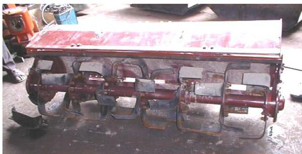
Fig 5 L-Shaped Blade for Upland Crop (Secondary Tilling)
