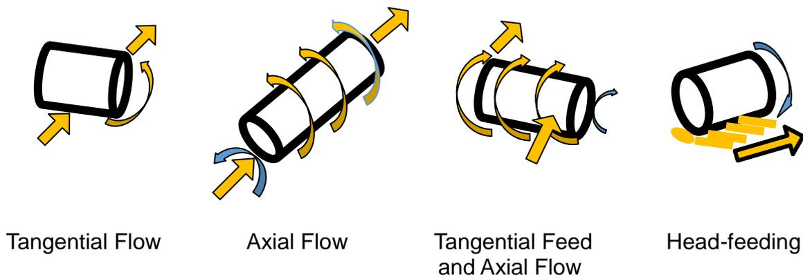
Fig. 11 Different feeding crops for various thresher
