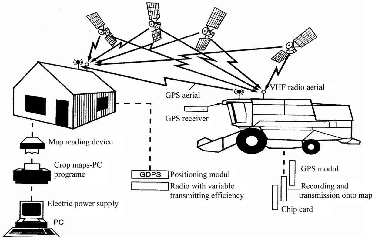
Figure 3. Global positioning system on the example of a combine harvester [7]
