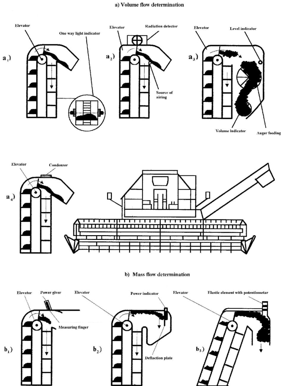
Figure 1. Systems for continual crop yield volume and mass flow determination
