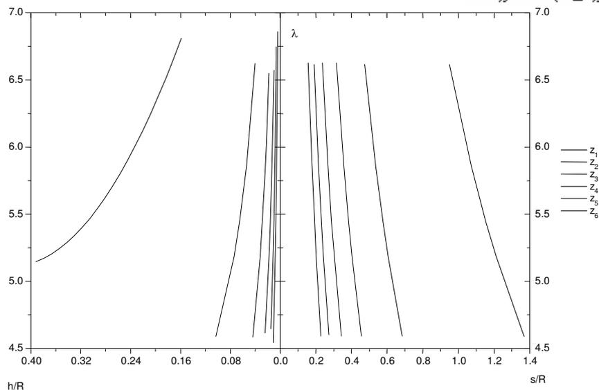
Fig. 4 – Variation of  $\lambda$  in relation with  $h/R$  and  $s/R$  (machine speed:  $v=4.8$  km/h)
