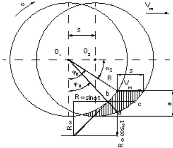
Fig. 1 – The parameters of the milling machine working process
