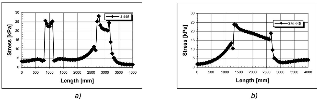
**Fig. 6.** Stresses distribution and graphical variation along the longitudinal direction to the top layer of the soil in longitudinal section for: a) U-445 tractor, b) SM-445 caterpillar tractor
