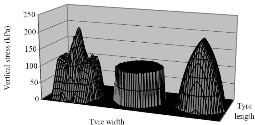
**Fig. 4.** Distribution of vertical load in the contact area [7]
