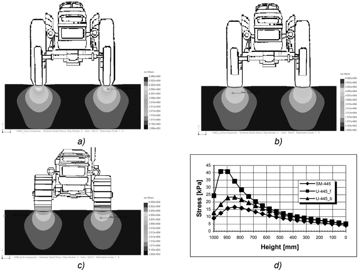
**Fig. 5.** Stresses distribution in cross-section for: a) front wheels of U-445 tractor, b) back wheels of U-445 tractor, c) SM-445 caterpillar tractor, d) graphical distribution along the axial-vertical direction
