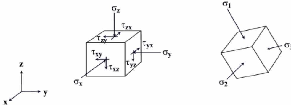
Fig. 2. Stress tensor components [8]
