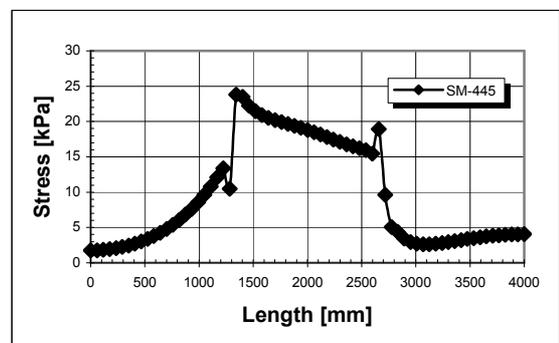
**Fig. 6.** Stresses distribution and graphical variation along the longitudinal direction to the top layer of the soil in longitudinal section for: a) U-445 tractor, b) SM-445 caterpillar tractor
