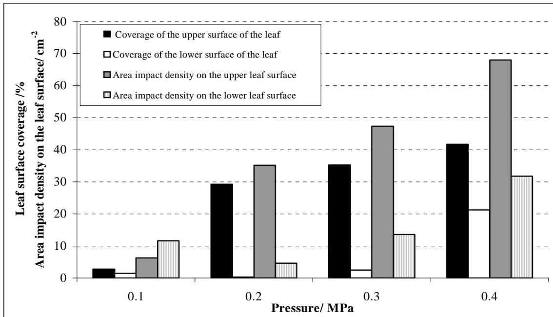
Fig. 6. Average coverage and area impact density on the upper and lower winter wheat leaf sides in case of the use of TeeJet 11006
