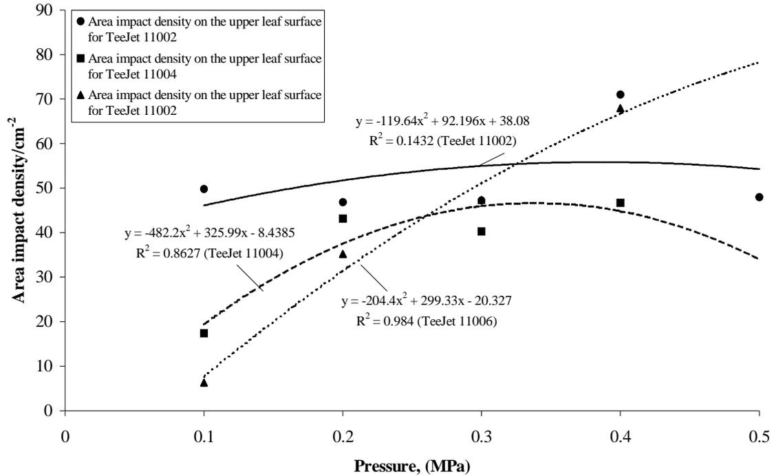
Fig. 9. Area impact density on the upper leaf surface for three nozzle types depending on the spraying pressure
