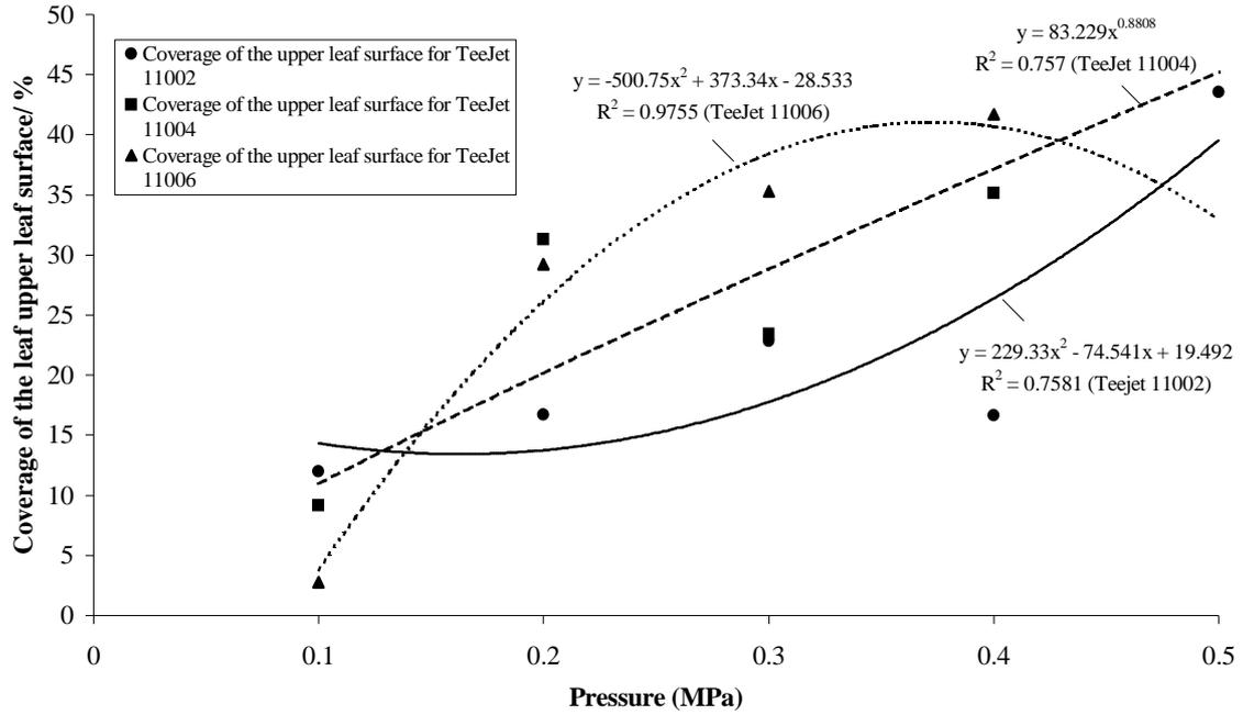
Fig. 7. Coverage of the upper leaf surface for three nozzle types depending on the spraying pressure
