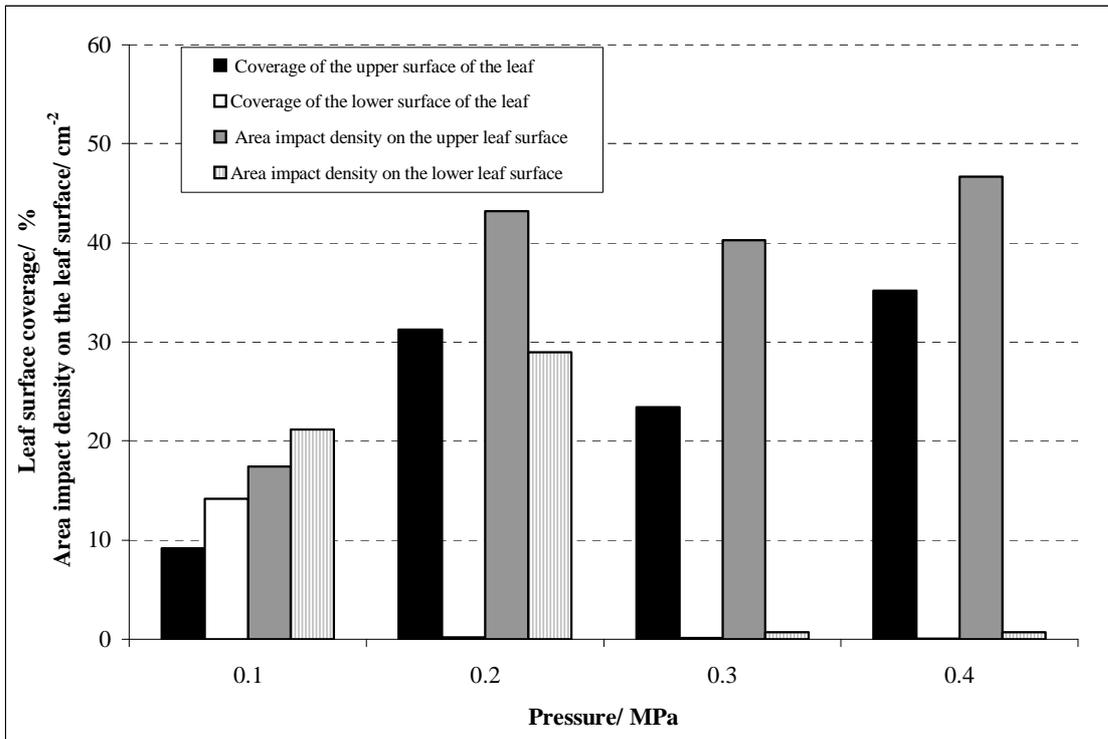
Fig. 5. Average coverage and area impact density on the upper and lower winter wheat leaf sides in case of the use of TeeJet 11004
