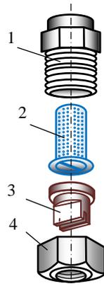
Fig. 2. a) Main parts of a TeeJet nozzle
