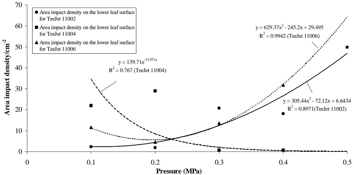
Fig. 10. Area impact density on the lower leaf surface for three nozzle types depending on the spraying pressure
