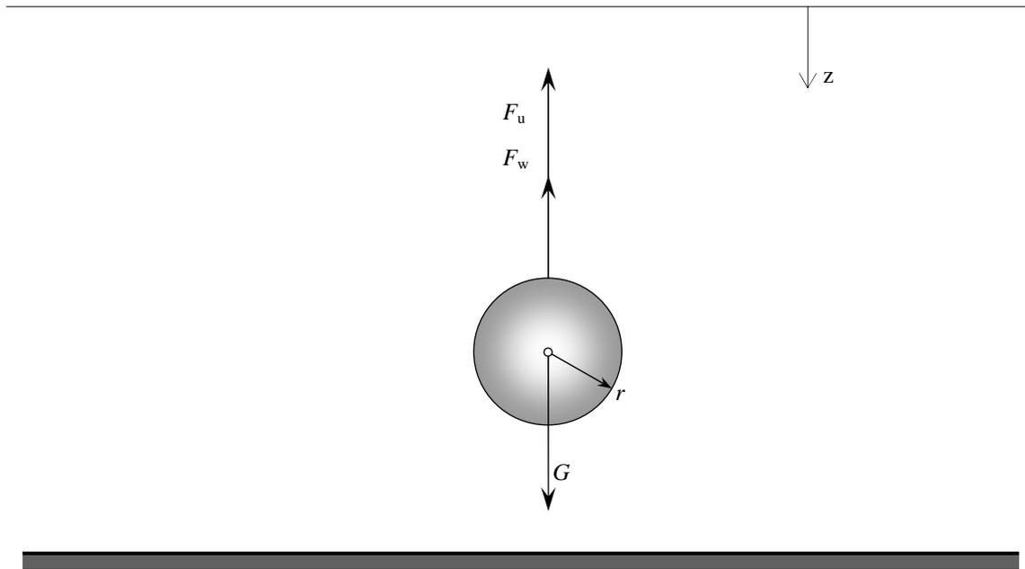
Figure 1. Spray droplet as a spherical model and forces acting upon it
