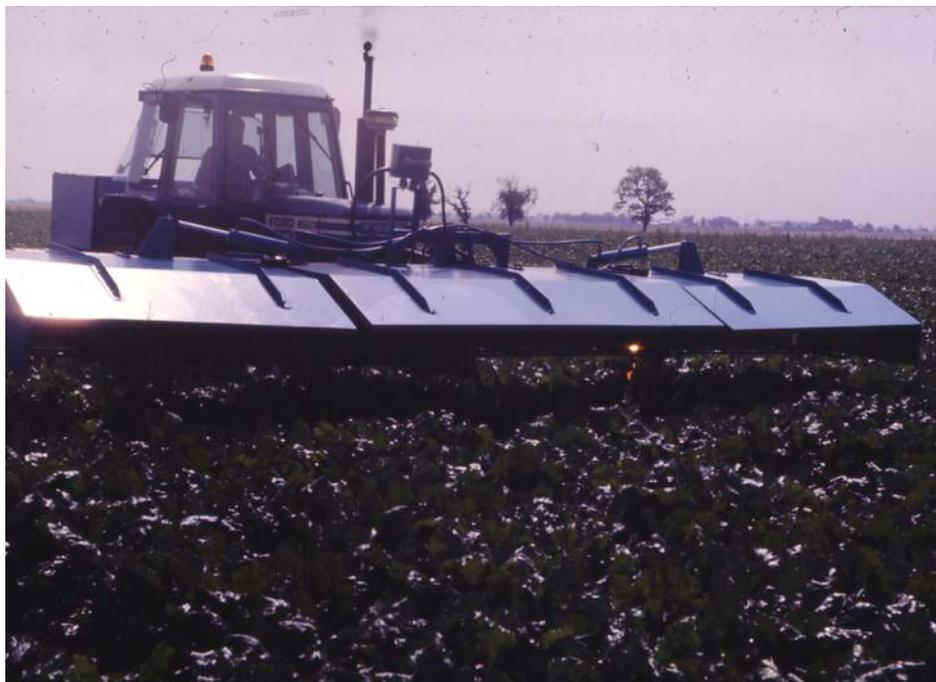
Figure 1: the British Sugar Corporation weed beet control machine developed in the 1980s
