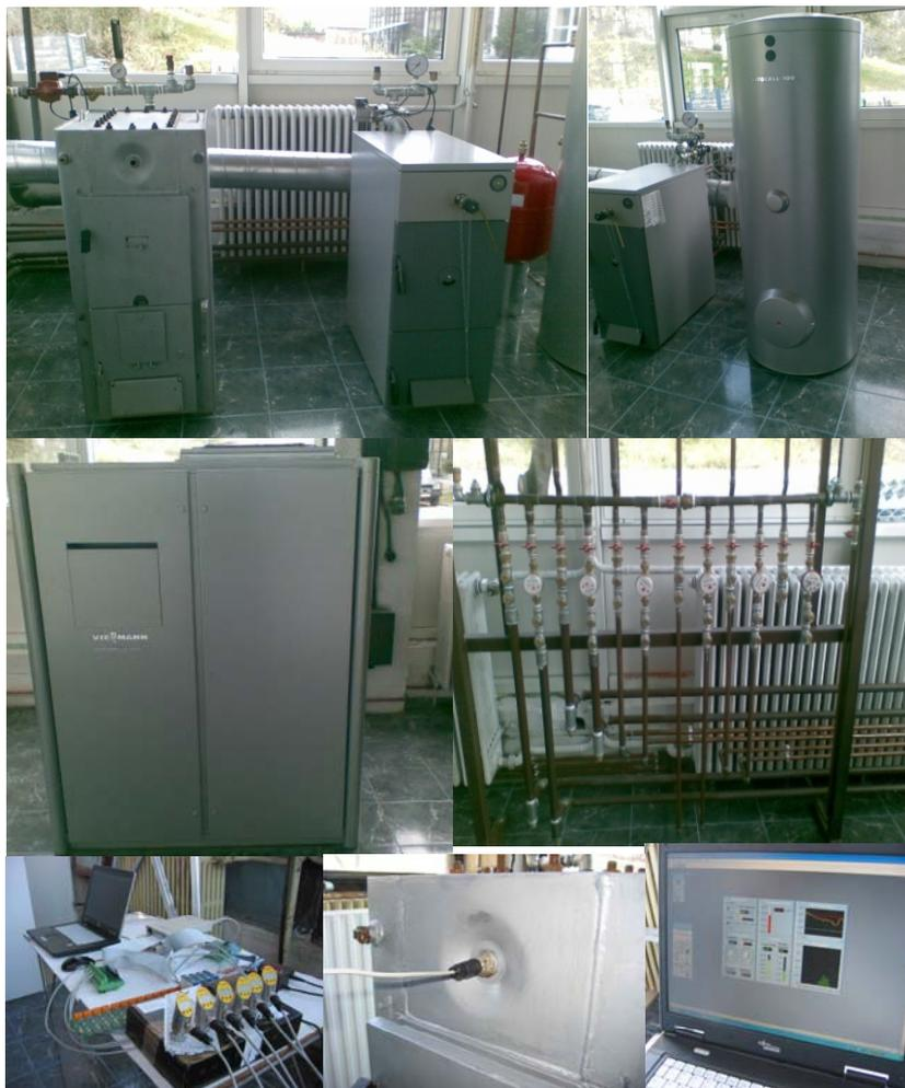
Fig. 3. The laboratory of Cogeneration Energy Based on Solid Biomass; a – solid biomass heating system; b – air – water heating system; c – data acquisition system for biomass heating system.
