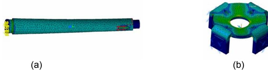
Fig. 6. stress distribution of Von Mises in sensitive components of the machine: (a) Shaft, (b) Shaft support.
