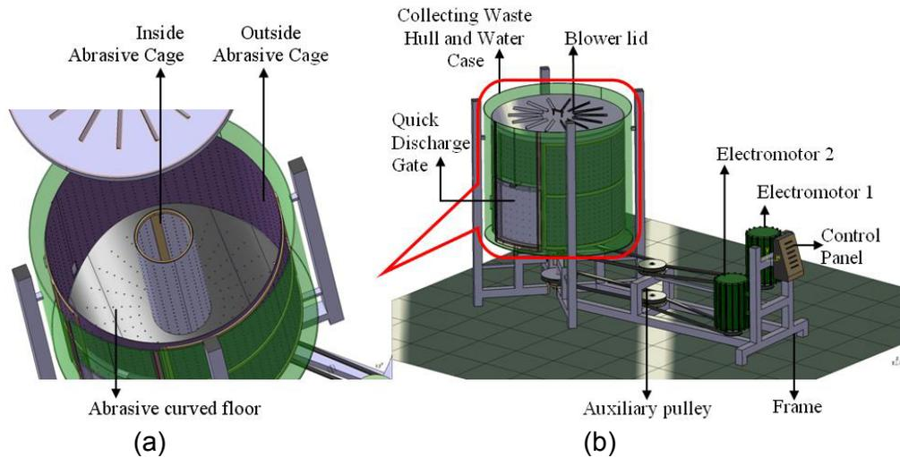
Fig. 2. General view of the proposed multipurpose machine: (a) Machine process chamber, (b) Different parts of the machine.
