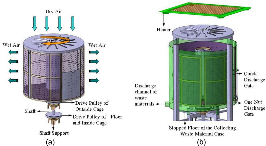
Fig. 4. (a) Drying operation method, (b) Different discharge channels.
