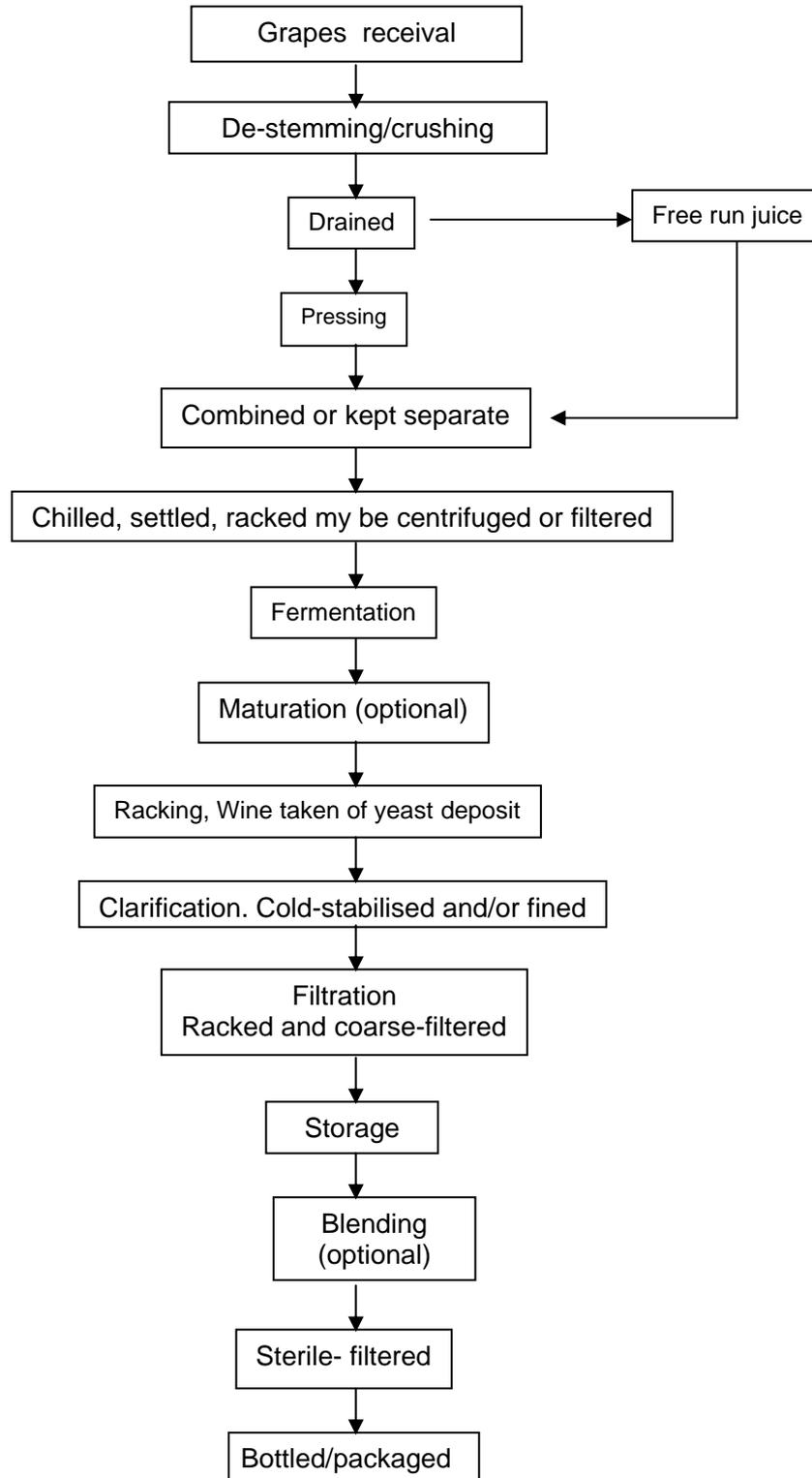
*Fig.1. The scheme of the technological process of grapes processing for producing white wines.*
