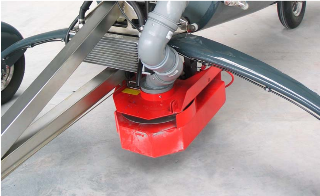
Figure 2. The centrifugal distributor for granules scattered with electric control. Photo: Pape
