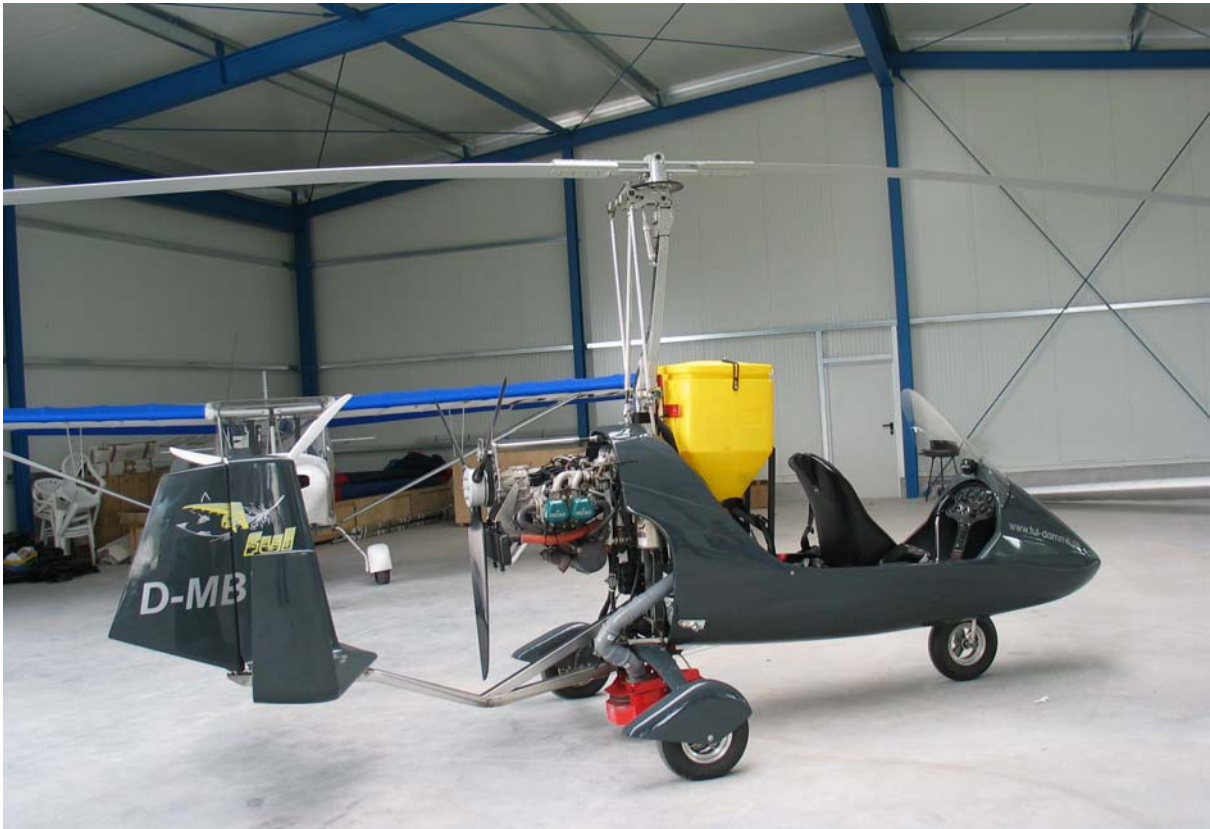
Figure 1. MT-03 gyrocopter fitted out with equipment for the granules Administration. Photo: Pape
