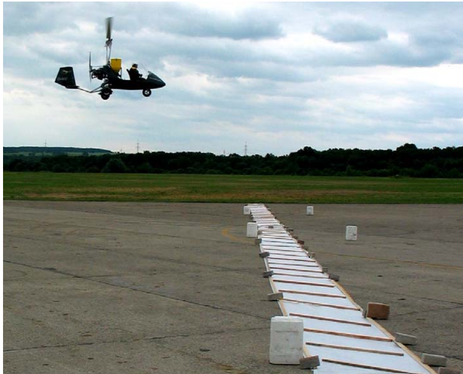
Figure 3. The distribution uniformity establishing of the granulated crop protection products.
