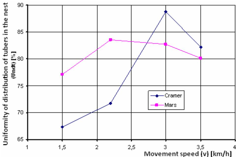
Fig. 4. Variation of uniformity of distribution of tubers into the nest at the two types of sections (CRAMER and MARS) depending on the working speed for the fraction 30...40 mm and the planting distance adjusted at 33 cm
