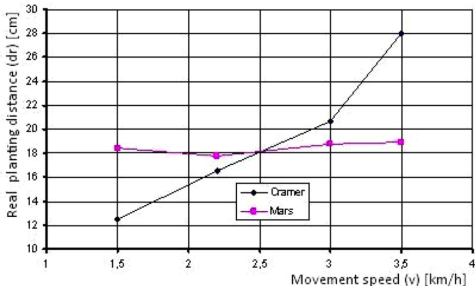
Fig. 3. Graphical representation of the real planting distance variation at the two types of sections (CRAMER and MARS) depending on the working speed, for round-shaped tuber from fraction: 30...40 mm and the planting distance set to 20 cm (CRAMER)/21 cm (MARS)
