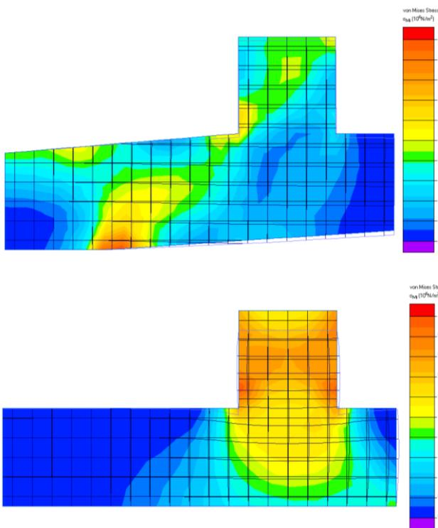
**Fig. 5.** Distribution of equivalent stresses in the adaptive tire in the contact area with the rolling track
