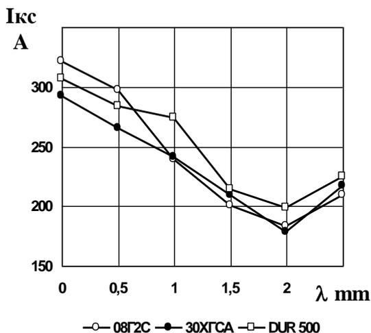
Fig.3. Impact of the amplitude of vibrations ( $\lambda$ ) on the short circuit amperage ( $I_{sc}$ ) during vibroarc weld overlay in Ar with different wire electrodes
