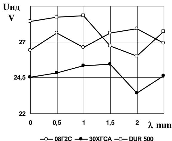
Fig.2 Impact of the amplitude of vibrations ( $\lambda$ ) on the voltage at the start of arc combustion ( $U_{start}$ ) during vibroarc weld overlay in Ar with different wire electrodes
