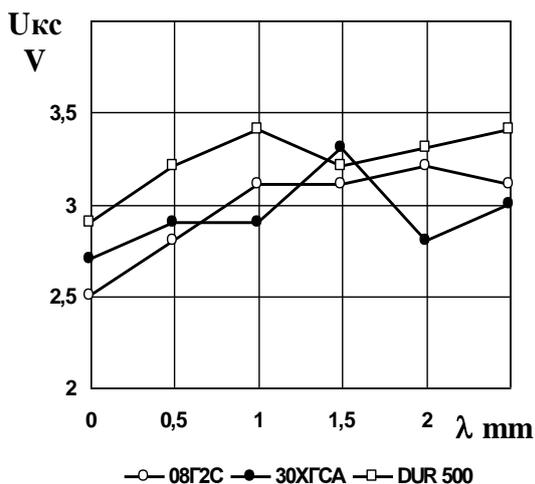
Fig.1. Impact of the amplitude of vibrations ( $\lambda$ ) on the short circuit voltage ( $U_{sc}$ ) during vibroarc weld overlay in Ar with different electrode wires
