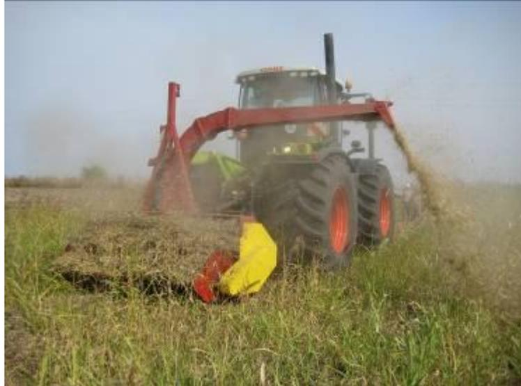
Figure 2. Hydroficated universal composting machine with a rotor cutting device
