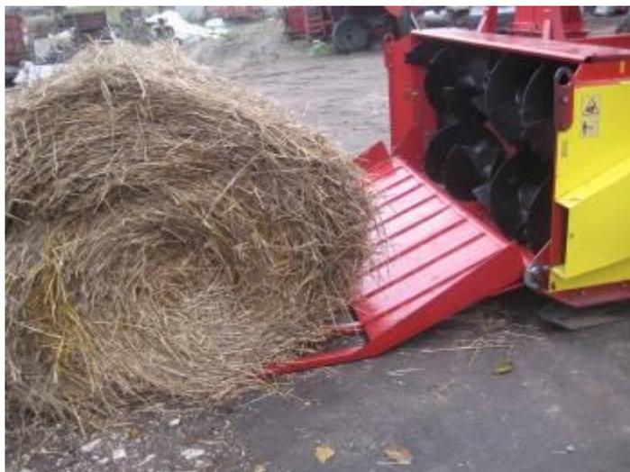
Figure 4. Hydroficated platform for crushing and shredding round and cuboid bales
