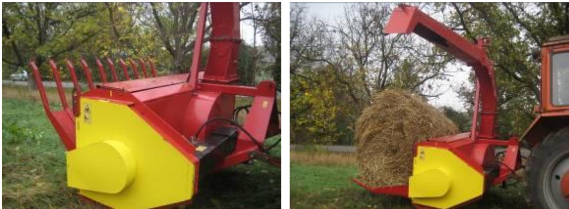
Figure3. Universal machine for composting with a hydroficated platform for crushing and shredding round and cuboid bales.
