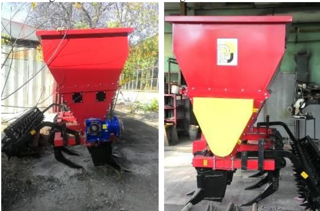
Figure 2. General view of the machine for importing organic matter in the soil
