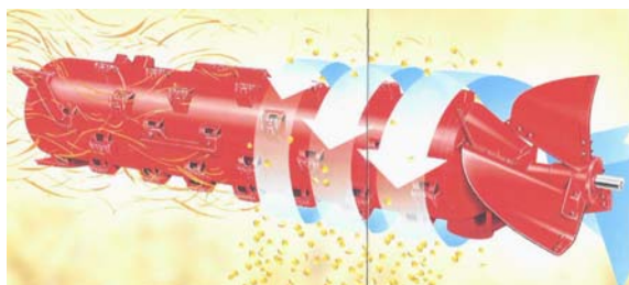
Figure 9 - Rotor of an axial thresher Case IH [6]
