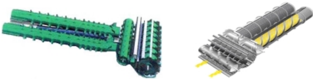
Figure 18 - Threshing apparatus with two axial rotors [6] a) John Deere 9780 CTS; b) Claas Lexion 480
