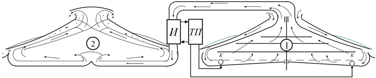
fig. 7. Energetical and manufacturing compatibility of the loops (1 – drying chamber, 2 – livestock building, TP – thermal pump, E – evaporator, K - condenser)
