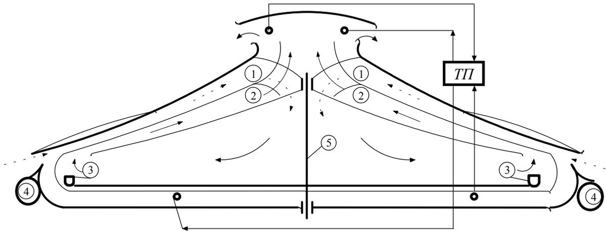
fig.3. Energy loop of energy-economical livestock building for floor breeding of animals and birds (patent [6] ) (TP –thermal pump, 1 – feeding channels, 2 – sucking channels, 3 – feeding facilities, 4 – bio generator chambers)
