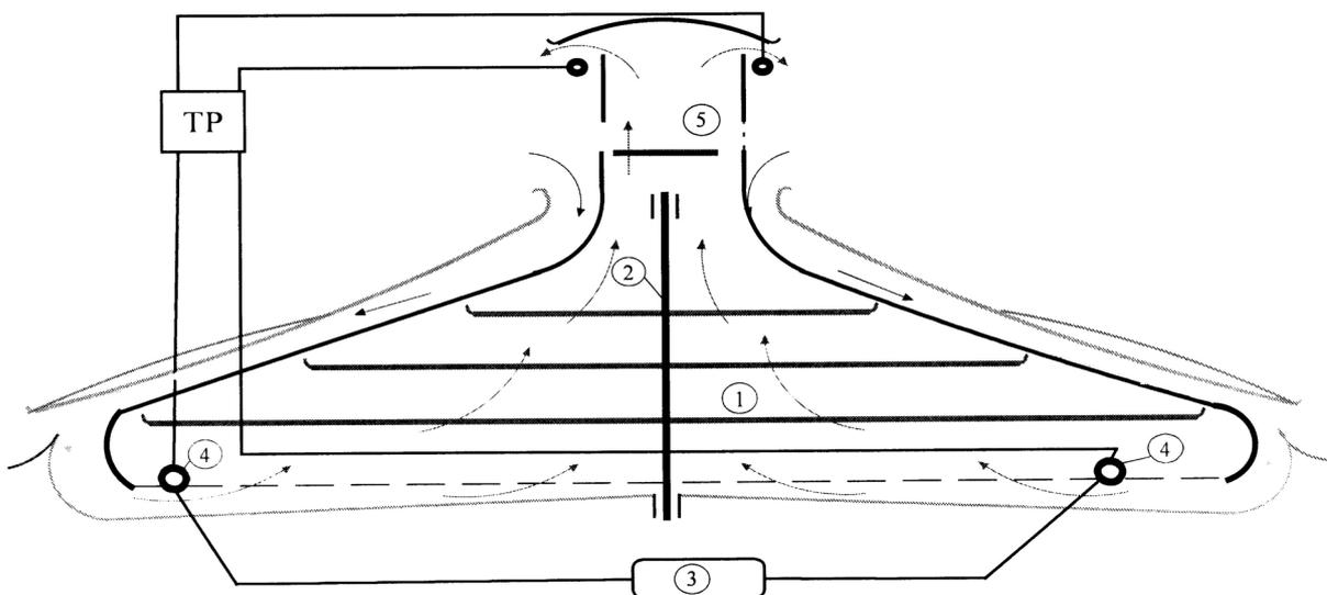
fig.6. Configuration and specific parameters for energy loop for fruit and vegetable dryer (patent [8]) (TP – thermal pump, 1 – working chamber, 2 – carrying axis and grids, 3 – boiler, 4 – heating serpentine)
