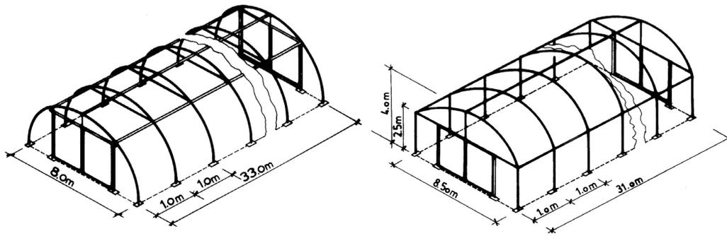
Figure 1. Quonset and arch type of greenhouses construction
