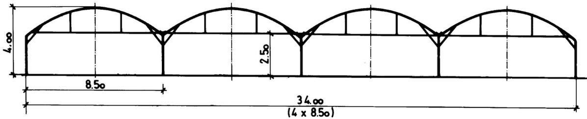
Figure 2. Multispan plastic covered greenhouse
