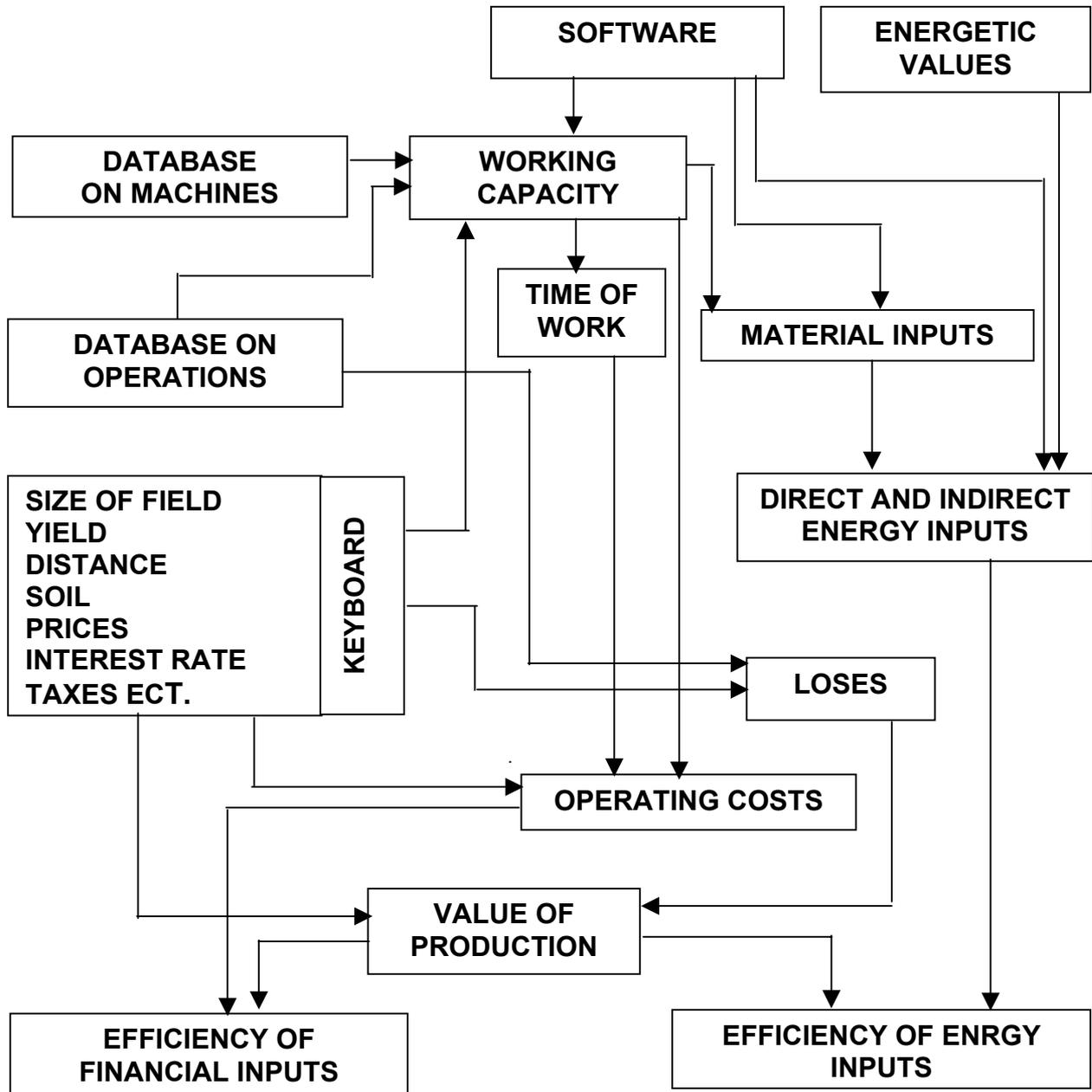
Figure 2. Scheme of the Decision Support System for biomass producers
