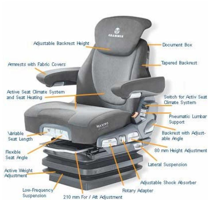
**Figure 2. A modern tractor seat with a pneumatic suspension system.**
