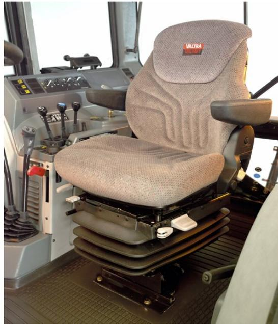
**Figure 12. A Valtra seat with Positive Response air suspension system.**
