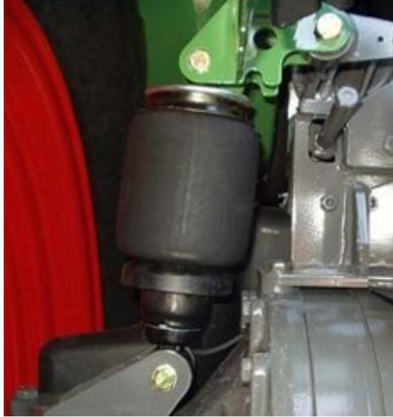
**Figure 8. The air spring shock absorber.**
