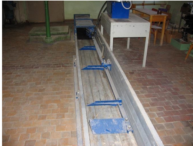
Figure 6. The device of the press manure removal, created for experiments by the idea of V. Veinla
